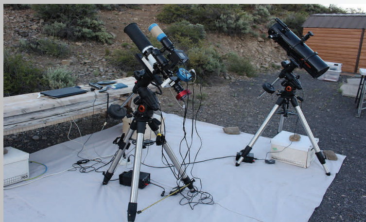
Fig. 1: Our original observing plan employed a 65mm refractor with a Shelyak ALPY 600 spectrograph. Observers were seated at picnic table on the north side of the telescope. The second instrument was a small Newtonian telescope for recreational visual observing during longer exposures.
